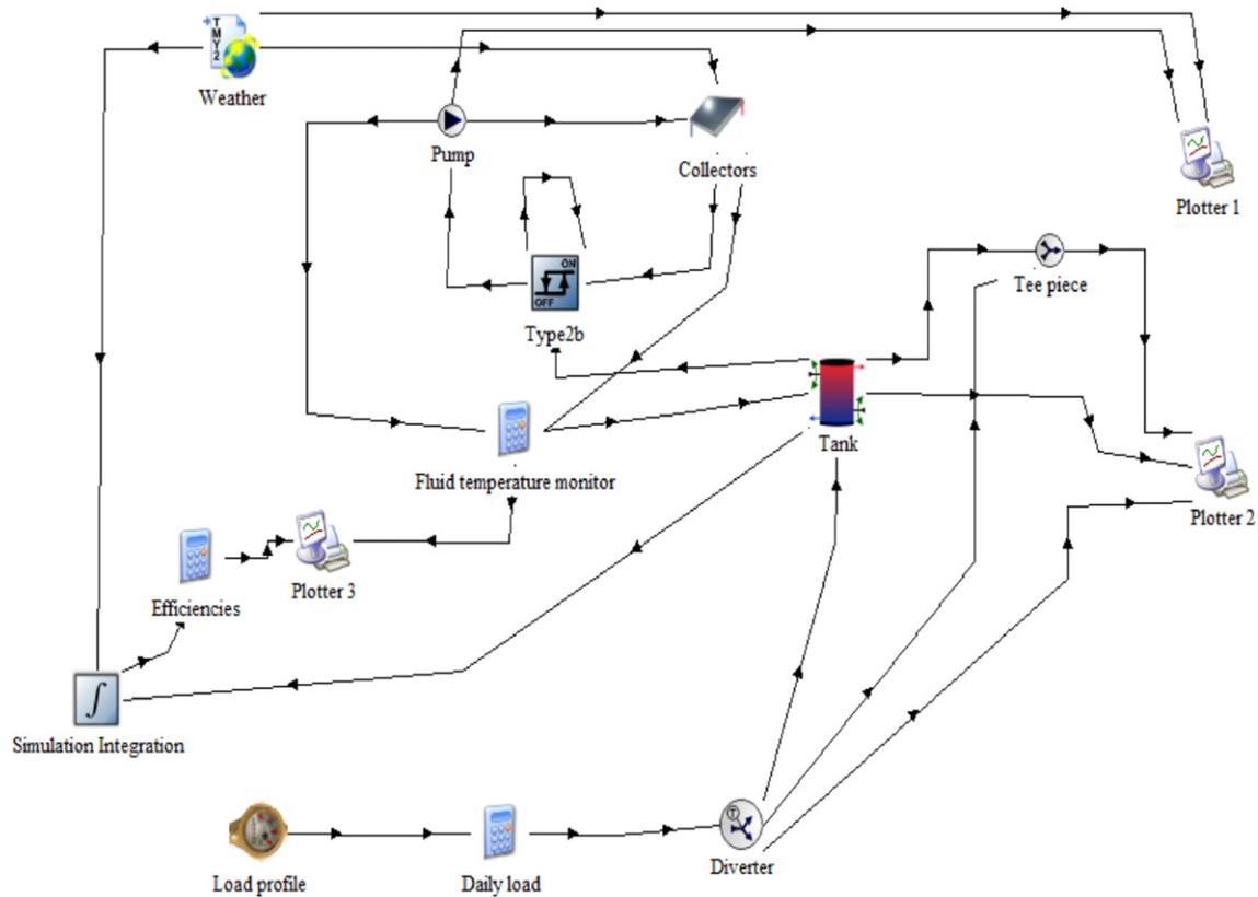
Fig. 5. The simulated SWH system in TRNSYS.
