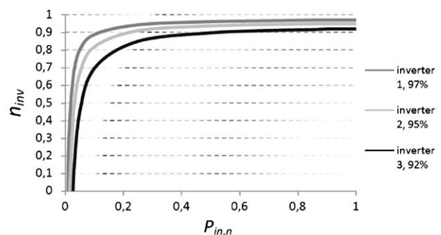
**Fig. 3.** Characteristic curves of the simulated inverters. The y-axis represents the inverter's efficiency ( $n_{inv}$ ) and the x-axis the ratio of the normalised power input to the inverter ( $P_{in,n}$ ).
