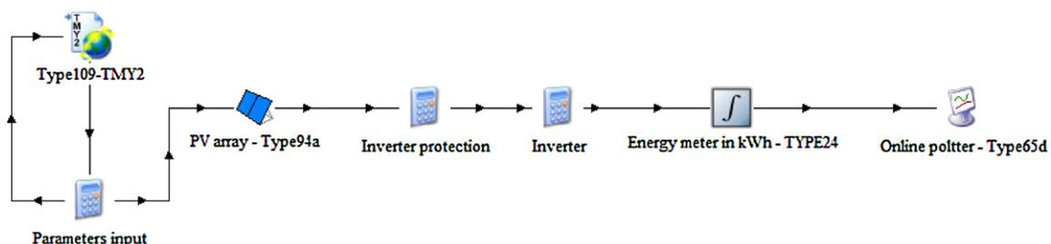
**Fig. 4.** The simulated circuit in TRNSYS-IIISiBat interface. The Inverter protection block cuts off any power values above the inverter nominal power. The Inverter equation block has been used instead of Type 135 to include the curves of Fig. 3, based on Eq. (2) of Ref. [33].
