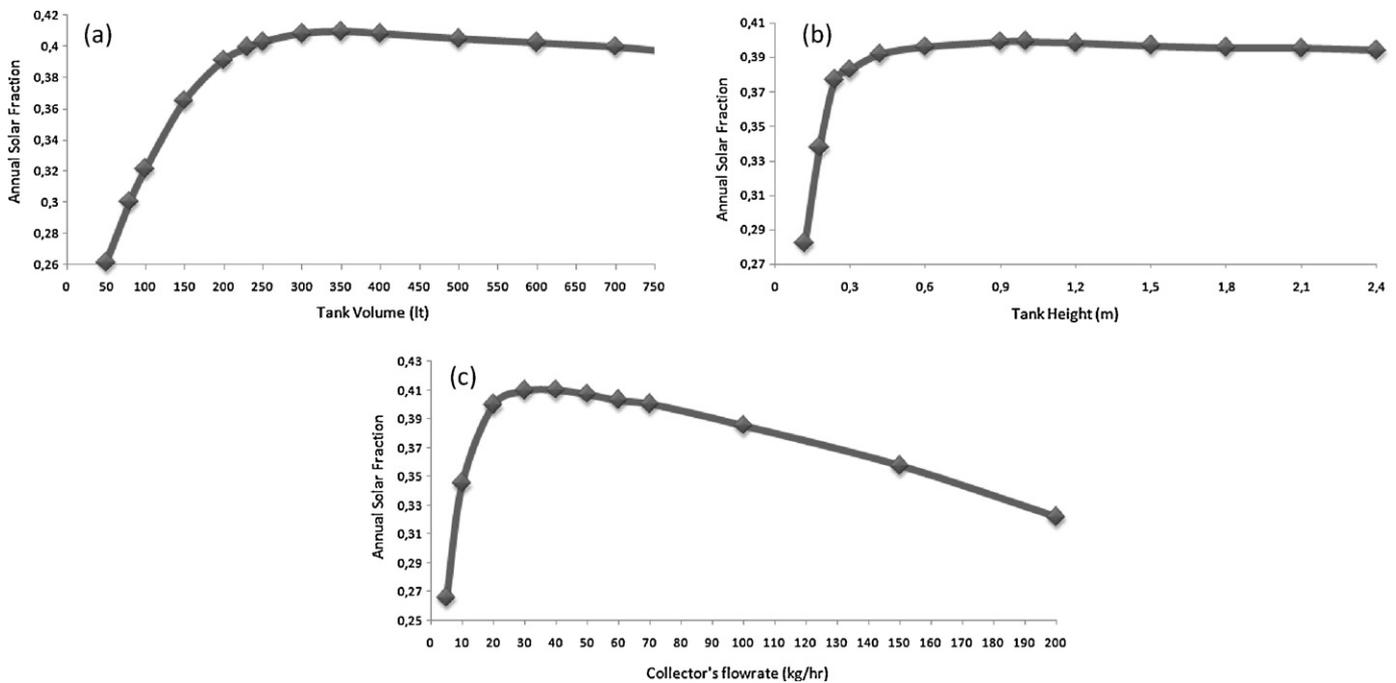
Fig. 7. Optimisation results for the SWH system: (a) optimal tank volume 350 L, (b) optimal tank height 1 m and (c) optimal flow rate 40 kg/h.
